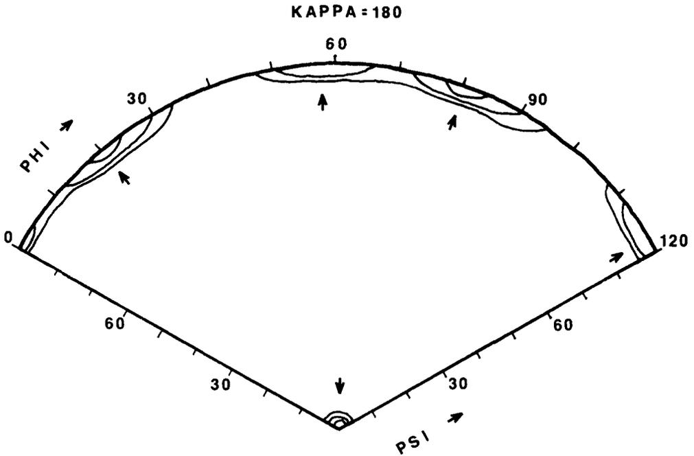
Fig. 3. The  $\kappa = 180^\circ$  section of the rotation function of the crystals of complexes between the gene 5 protein and d-(GGTAAT). All of the peaks along  $\psi = 90^\circ$  are of high magnitude with respect to the crystallographic symmetry peak, and all represent local, noncrystallographic symmetry elements present in the crystals.
